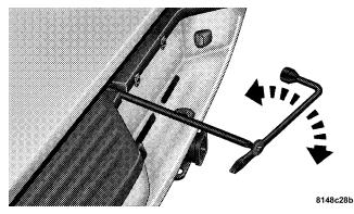
**Turning Lug Wrench and Extension** It is recommended that you stow the flat or spare to avoid tangling the loose cable.
